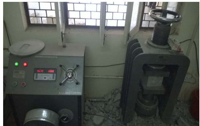
Fig. 6: Compressive strength test in progress
