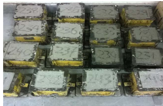
Fig. 3: Concrete Cubes made with different proportions of Iron Slag
