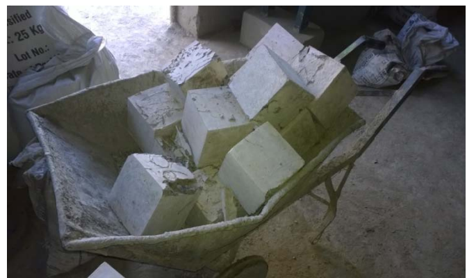
Fig. 7: Concrete cubes after compression testing
